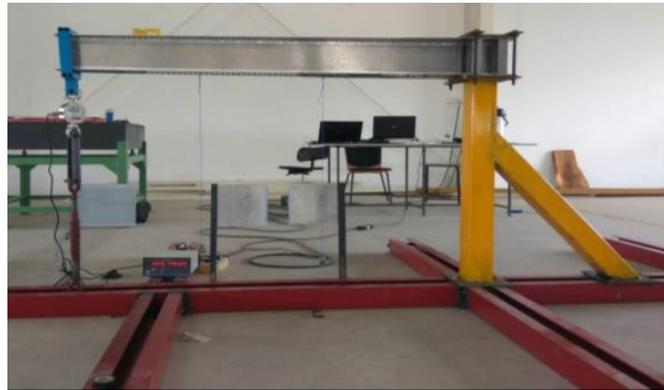
**Fig. 6 Test rig with spar**
