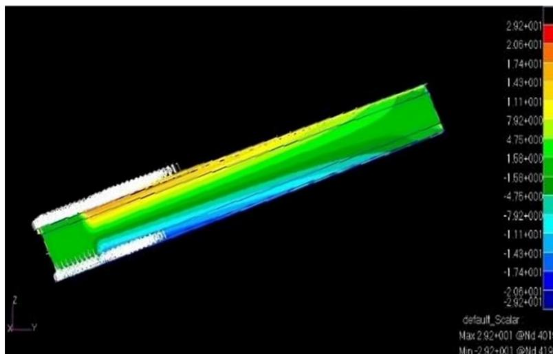
**Fig. 5 Maximum stress of the spar**
