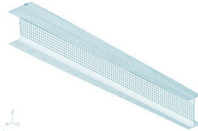
**Fig.2 Meshed spar model**
